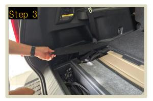
After removing the floor trim, you can detach the side panel to reach the area for the center hole template.
