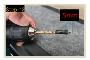
Ready the 9mm drill bit, marking it 5mm from the tip to prevent drilling into any metal or components behind the side trim.
