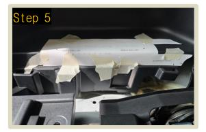
The center hole template should now be correctly placed.
