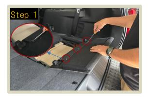
Detach the clips securing the floor trim on both sides.
