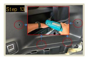
Drill holes in the locations shown, using an angle drill with a 9mm drill bit..
