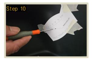
Repeat the marking process with a center punch for the right hole template, indicating the drilling spot.
